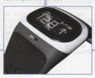
by Liz Dickenson, this product uses revolutionary electro-optical technology that shines a light through the skin in the wrist and measures the impedance - or interruption - of that light in order to read athletes' heart rates. This extraordinarily unique technology has been proven to be ECG (electrocardiogram) accurate at running speeds up to 12-20 mph.
